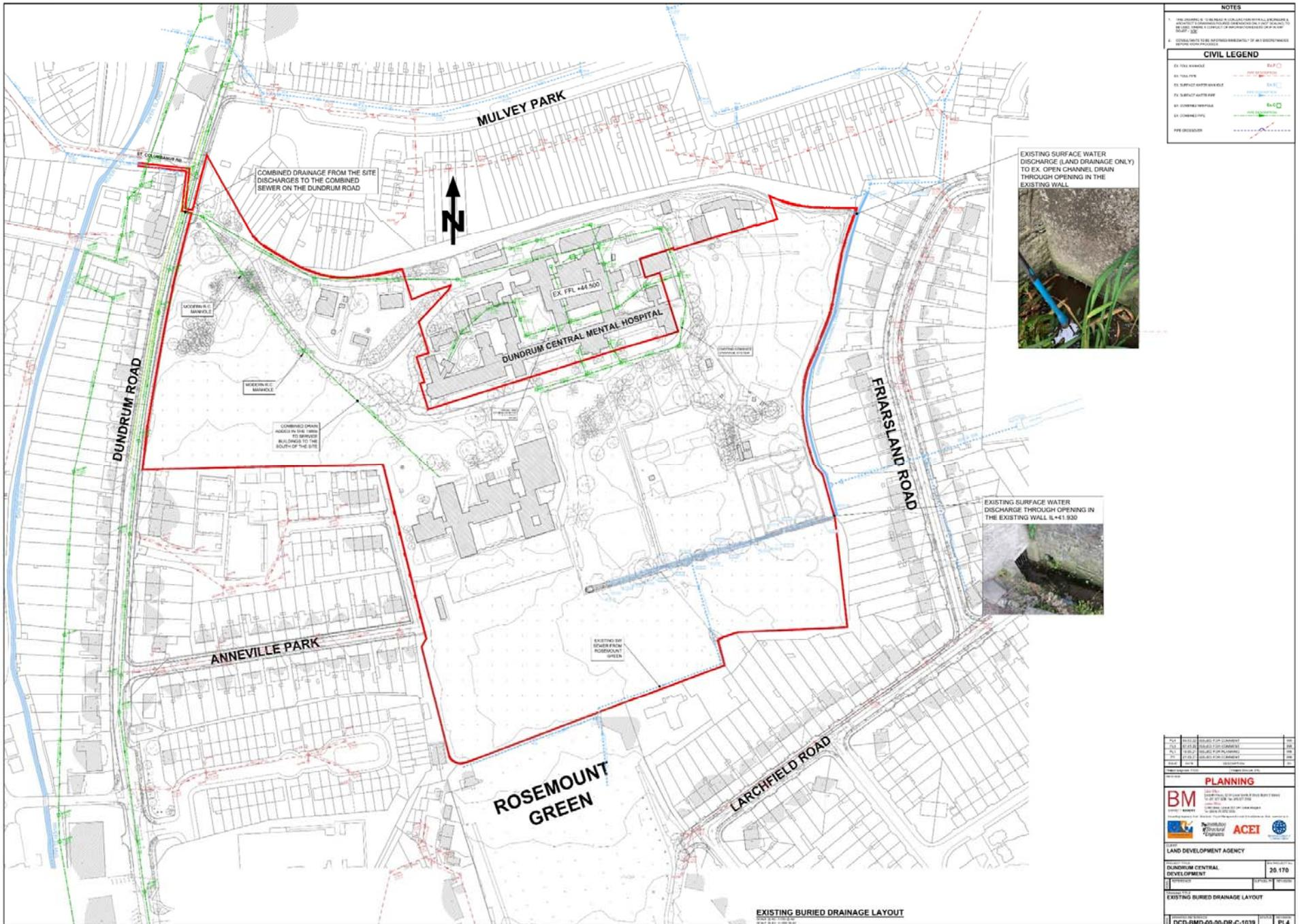
Figure 6. Existing surface water drainage layout
