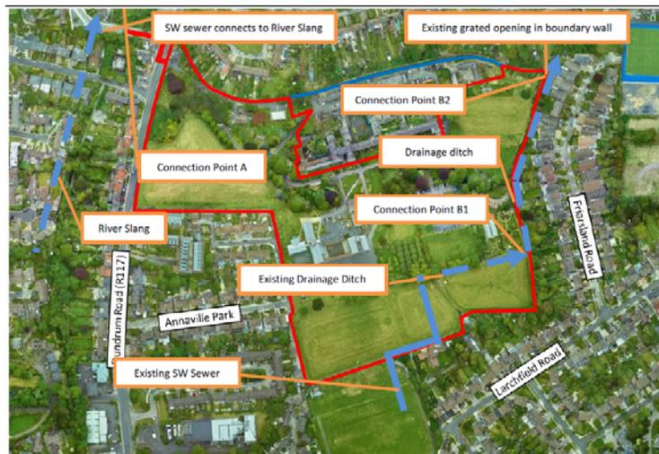
Figure 2.1 - Aerial view of the site with two surface water drainage connection locations indicated.
